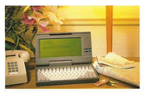
The Data General WALKABOUT™ portable terminal is a multi-purpose, industry-compatible, battery-powered terminal that fits easily into a briefcase. This compact terminal weighs only five pounds, and features a tiltable, easy-to-read, 25-line, supertwist liquid crystal display (LCD) screen and full-size keyboard.
