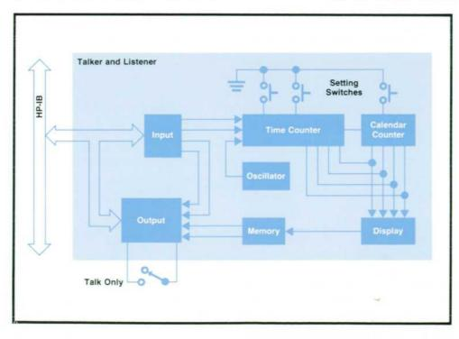
Fig. 3. Model 59309A ASCII Digital Clock is settable by frontpanel and remote control.
