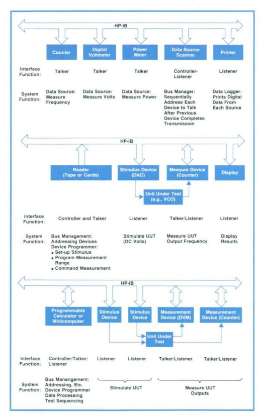
Fig. 2. Addition of a scanner enables several measurement devices to take turns supplying data to a recording device.
