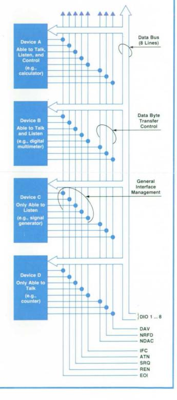
needed to interconnect a wide range of products from which systems can be configured with a minimal amount of additional engineering. Although it facilitates the assembly of systems, it does not guarantee the assembly of "instant" systems. Configuring a complete operating system demands detailed attention to all the device-dependent characteristics beyond the scope of the HP Interface Bus definition.
