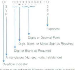
Inclusion of an indication of measurement units is especially useful with multifunction modules, such as the Model 5306A Multimeter (volts, ohms, frequency).
