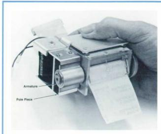
Fig. 3. Print mechanism is uncomplicated.
