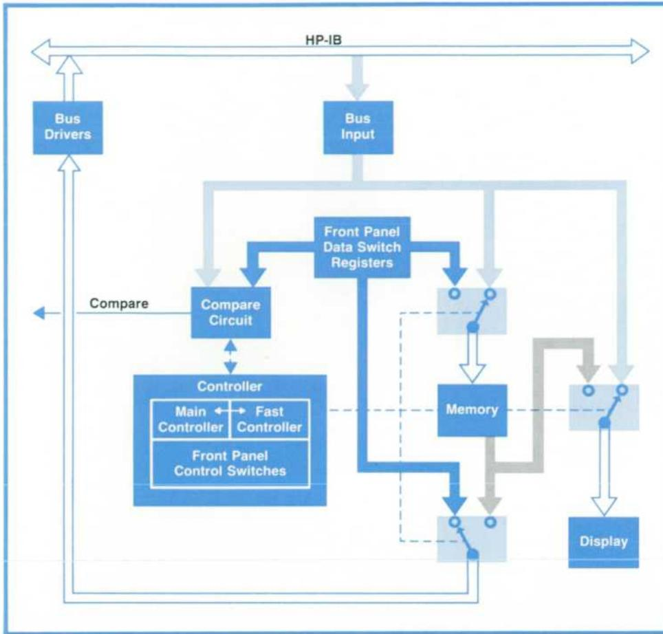
**Fig. 3.** Simplified block diagram of the Model 59401A Bus System Analyzer. The switches shown represent gates operated in combinations by the internal controller in response to front-panel switch settings. The main controller manages most operations but a fast bipolar controller is used for the FAST TALK and FAST LISTEN functions.
