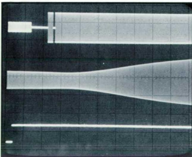
**Fig. 2.** Oscilloscope demonstrates use of the bus analyzer as an oscilloscope trigger (see text). The bottom trace shows the timing of the analyzer's "compare" pulse. The top trace shows the synthesizer output in response to the trigger event and the middle trace shows the output of the filter under test.
