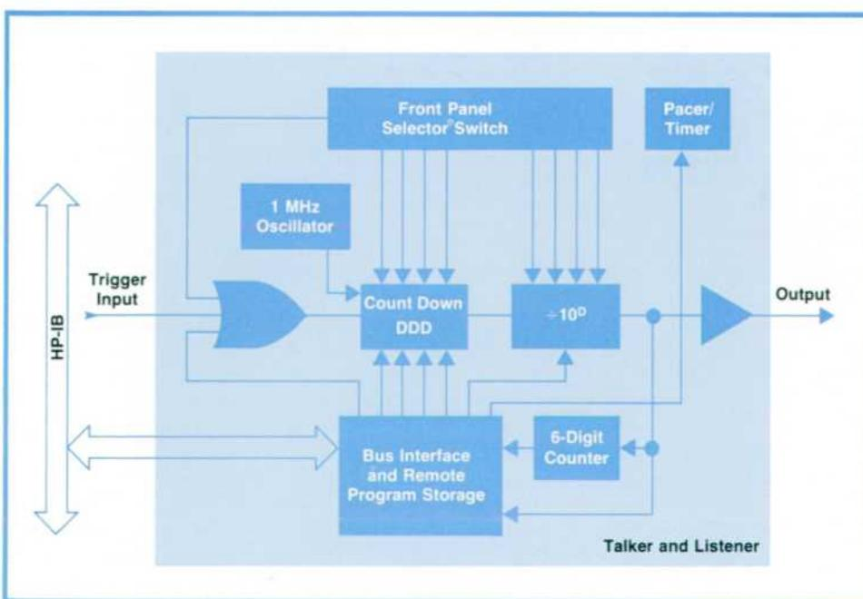
Fig. 2. Model 59308A Timing Generator functions as a digital delay, a time mark generator, and a time-interval counter.
