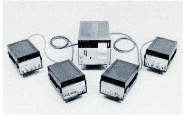
face bus only when addressed by the controller. If the timing of a measurement is important, such as several inputs to be measured simultaneously, an initiate command directs each instrument to take a reading and hold it until addressed to put the data on the bus. When used with a desk-top calculator or a computer, the modules provide a low-cost approach to multiple-input data acquisition systems that can be modified any time with more complex instruments without modifying the interface.
