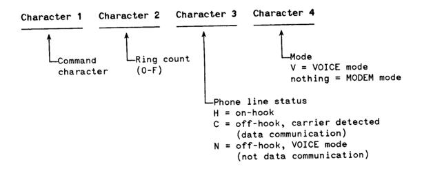
Any parameter or mode changes are executed after the command string is terminated. Therefore, multiple Q commands in a command string will usually be redundant. The only exceptions are commands that alter the on-hook/off-hook state, since they are executed as they appear in the command string. If multiple Q commands are intertwined with those commands, the responses will reflect the status of the modem at the time each Q is executed.
