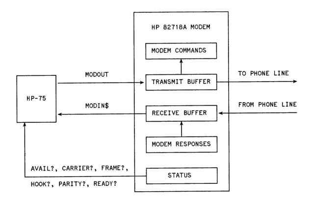
When MODOUT sends a string from the HP-75 to the modem, it places the string in the 8-byte modem transmit buffer. The modem then examines the transmit buffer to see what action it should take. If the
