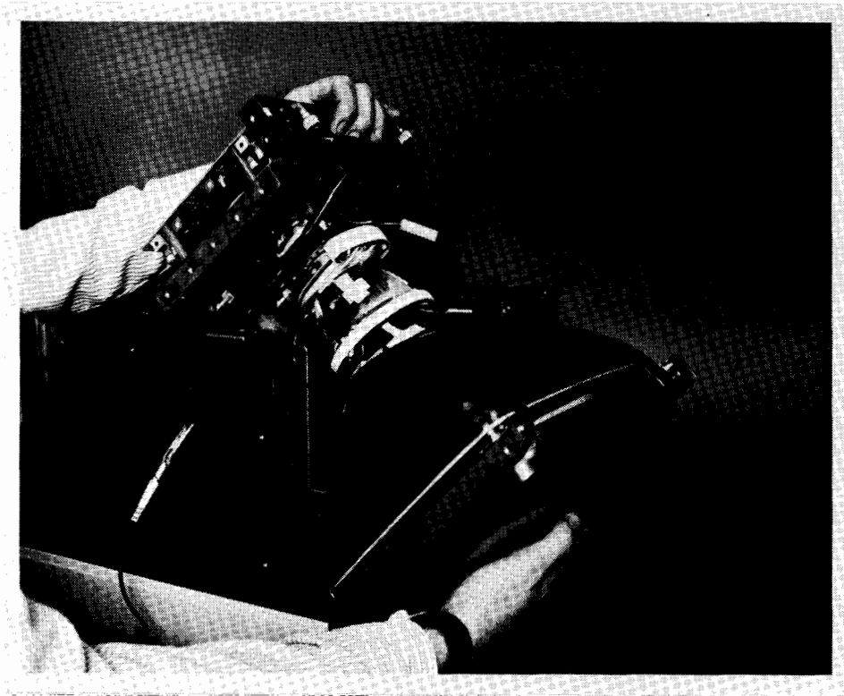
Figure 4-17. Removing the Video Board/CRT Unit.
