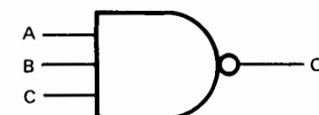
DENOTES "NAND" GATE: "AND" WITH INVERTED OUTPUT.
