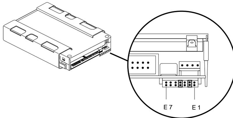
**Figure C-1** Floptical Drive Jumpers Set to SCSI Address 2
