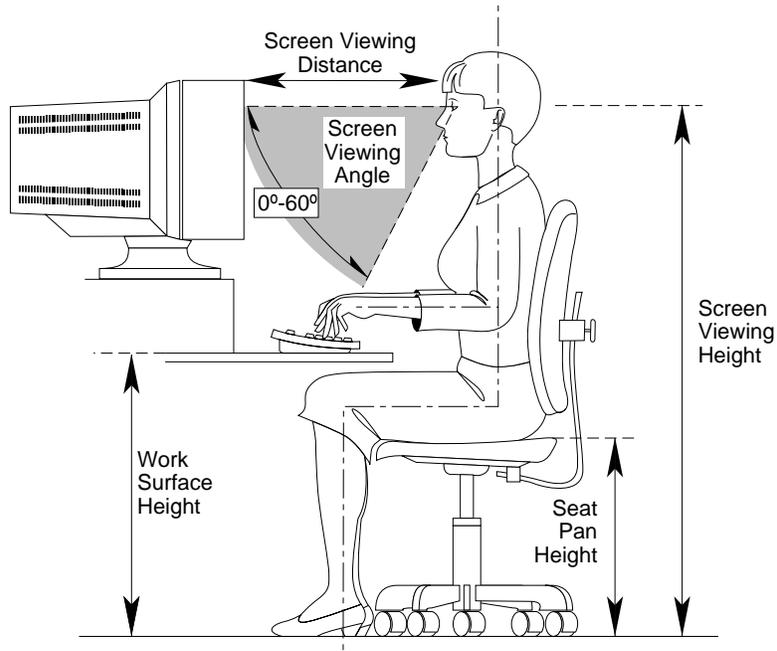
**Figure 9-1** Basic Parameters of Visual Display Terminal Workstation Adjustment (Adapted From ANSI/HFS 100-1988)
