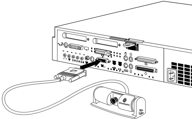
**Figure 2-19** Connecting the IndyCam Camera Cable to the Workstation
