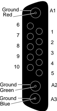
Figure A-13 Graphics Port Pinout Assignments
