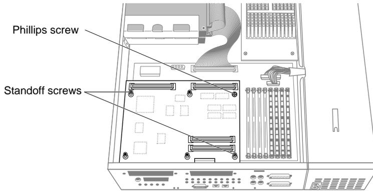
**Figure 8-12** Inserting the Screws on the Graphics Board
