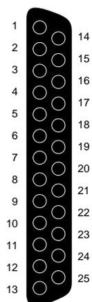
**Figure A-3** Parallel Port Pinout Assignments
