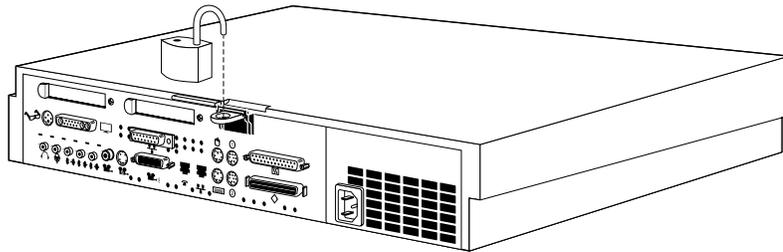
**Figure 2-30** Attaching a Lock to the Indy Workstation
