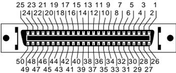
**Figure A-9** SCSI Port Pinout Assignments
