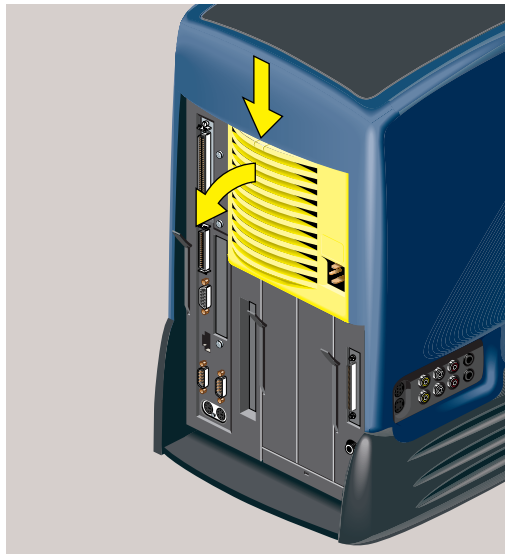
Figure 5-37 Removing the Bezel From the Power Supply
