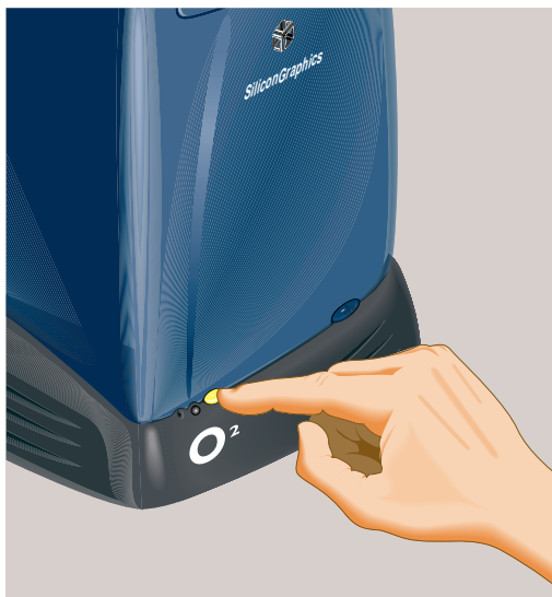
Figure 2-1 Turning Off the O2 Workstation
