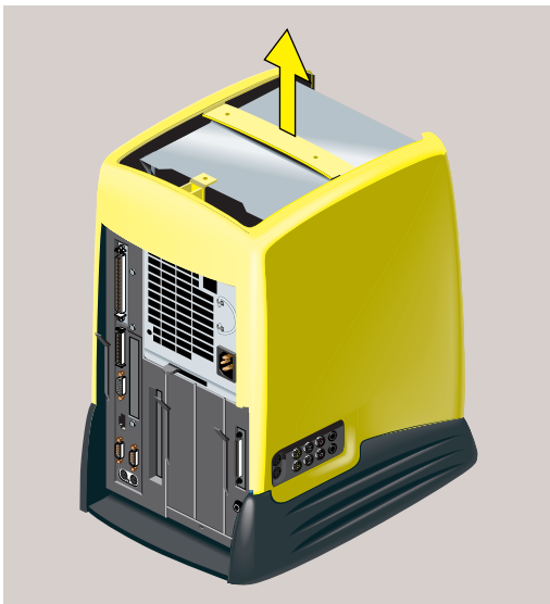
Figure 5-49 Removing the Outer Cover
