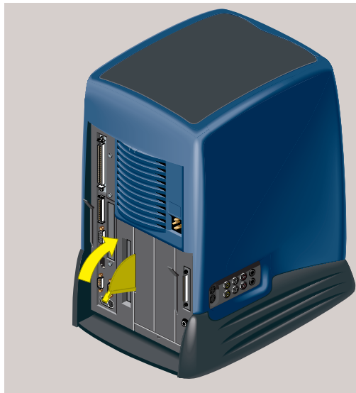
Figure 5-25 Securing the System Drive Module
