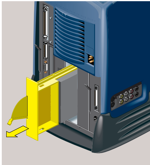
Figure 5-23 Removing the System Drive Module From the Chassis
