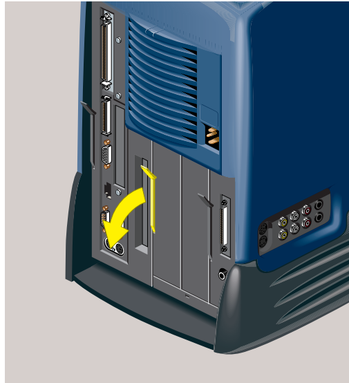
Figure 5-22 Releasing the Drive Tray
