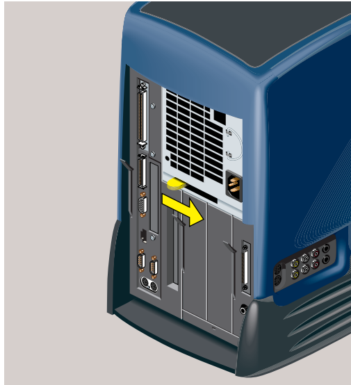
Figure 5-38 Releasing the Power Supply
