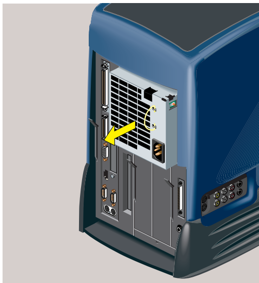
Figure 5-39 Removing the Power Supply From the Chassis
