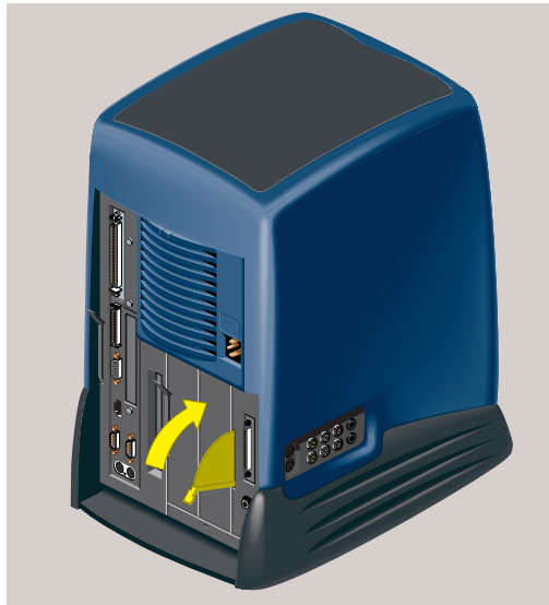
Figure 3-10 Securing the Audio-Visual Module
