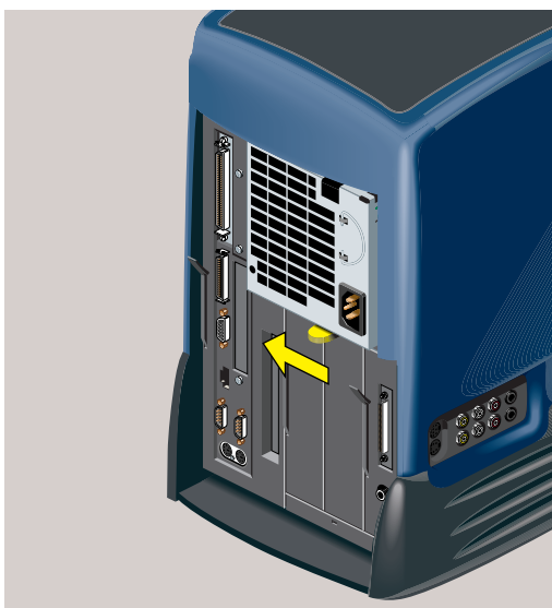
Figure 5-41 Locking the Power Supply in Place
