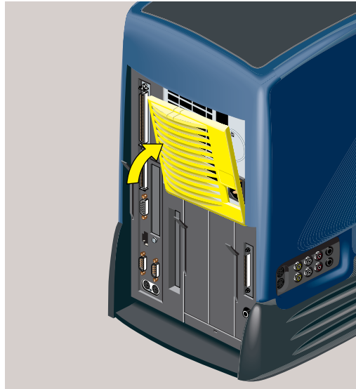
Figure 5-42 Replacing the Bezel on the Power Supply
