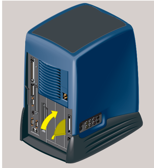
Figure 5-32 Securing the Audio-Visual Module
