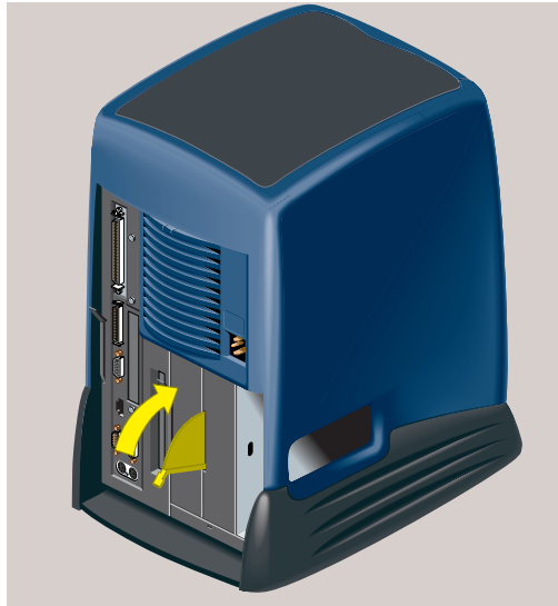
Figure 3-8 Securing the Second Hard Drive Module
