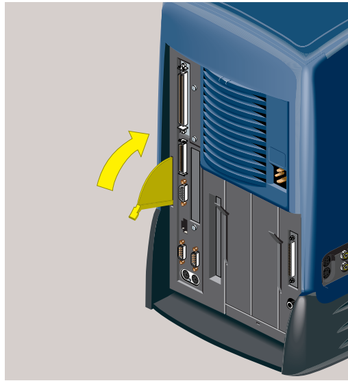
Figure 2-48 Securing the System Module in Place
