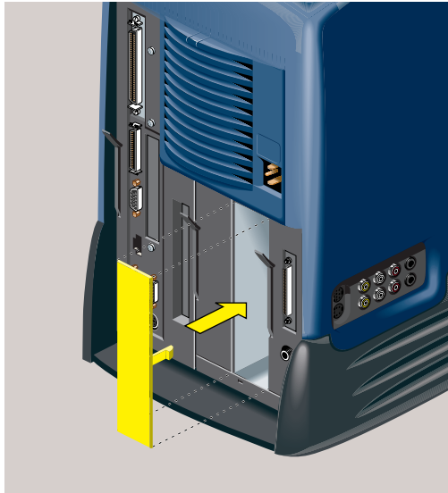
Figure 3-16 Replacing the Filler Panel
