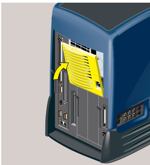
Figure 5-59 Replacing the Power Supply Bezel
