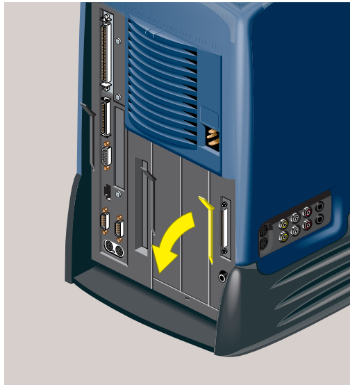
Figure 3-4 Releasing the Audio-Visual Module
