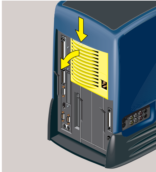
Figure 5-46 Removing the Power Supply Bezel
